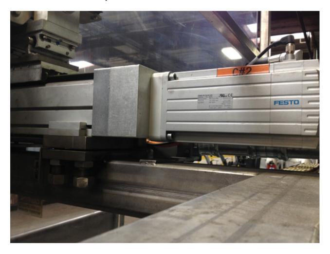
With such mass and weight, accuracy, repeatability, and safety become essential qualities. On that front, CoDeSys soft motion software is used to synchronize two Festo electric linear guides—actuated by servo-controlled motors—to run in parallel. Servo-controlled motion is far more accurate and repeatable than the previous mechanical chain-sweep system.
