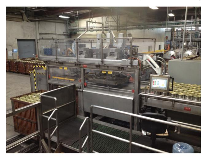
Filled soup cans are placed into baskets that can weigh hundreds of pounds, which are then manually loaded into horizontal steam retorts. After the retort process culminates, the loaded baskets are placed on a conveyor that leads to a basket unpacking station. Then, at this point, the cans are moved onto a labeling and case-packing line.
